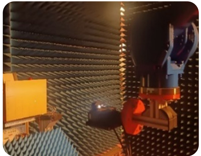
5 - Alignment setup with camera
