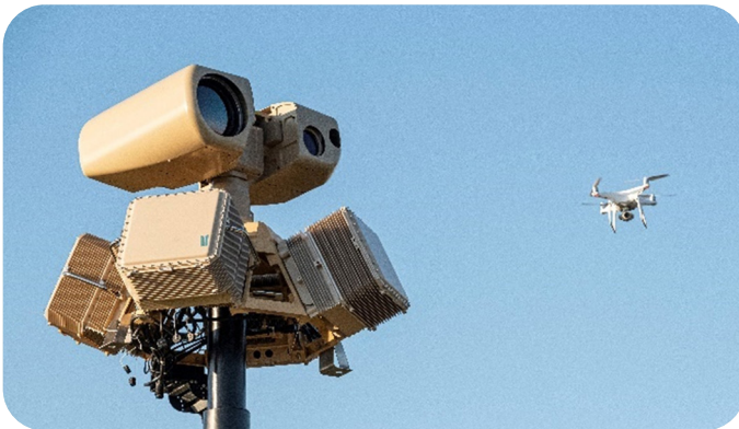
4 – Integrated Multifunctional Radar and Optical Sensors on an extendible mast for Surveillance and Counter-Drone Missions
