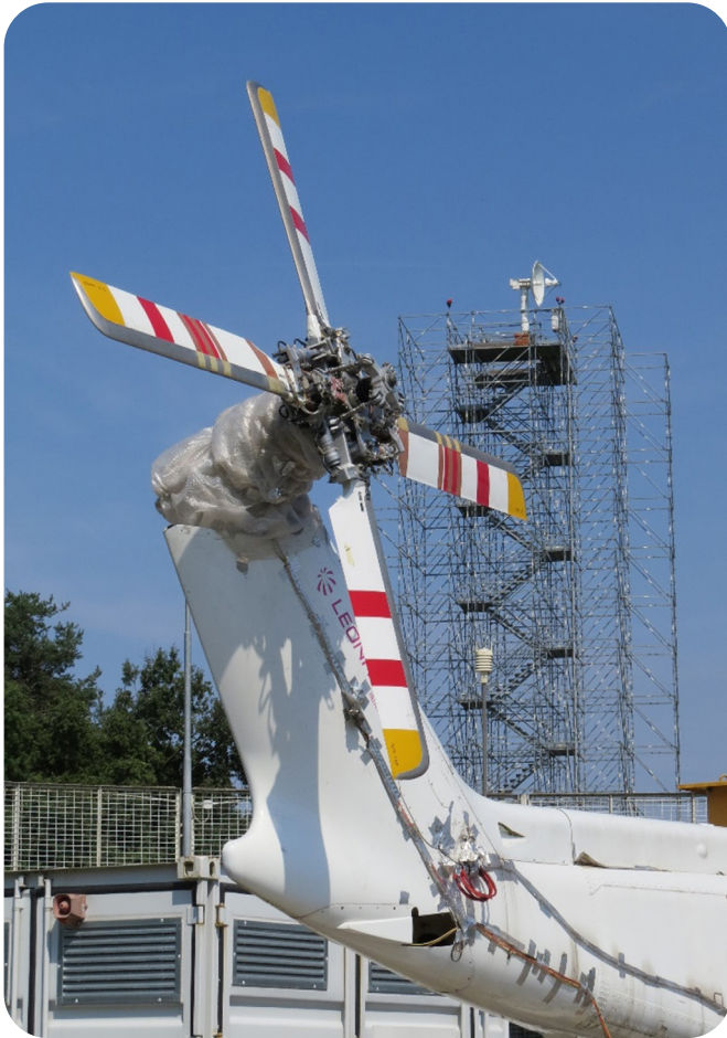
4–One of the tower-mounted telemetry antennas at Cascina Costa airfield, in the background of an instrumented tail rotor test rig
