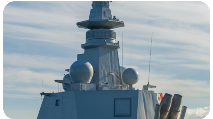
5-Shipborne Conformal Radar Antennas (Square Faces for Primary Radars and toroidal Secondary Radar antenna on top)
