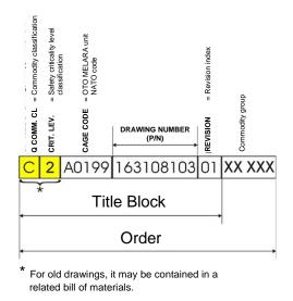
Figure 1 - Example of built-to-drawing item designation (OTO Melara La Spezia)
