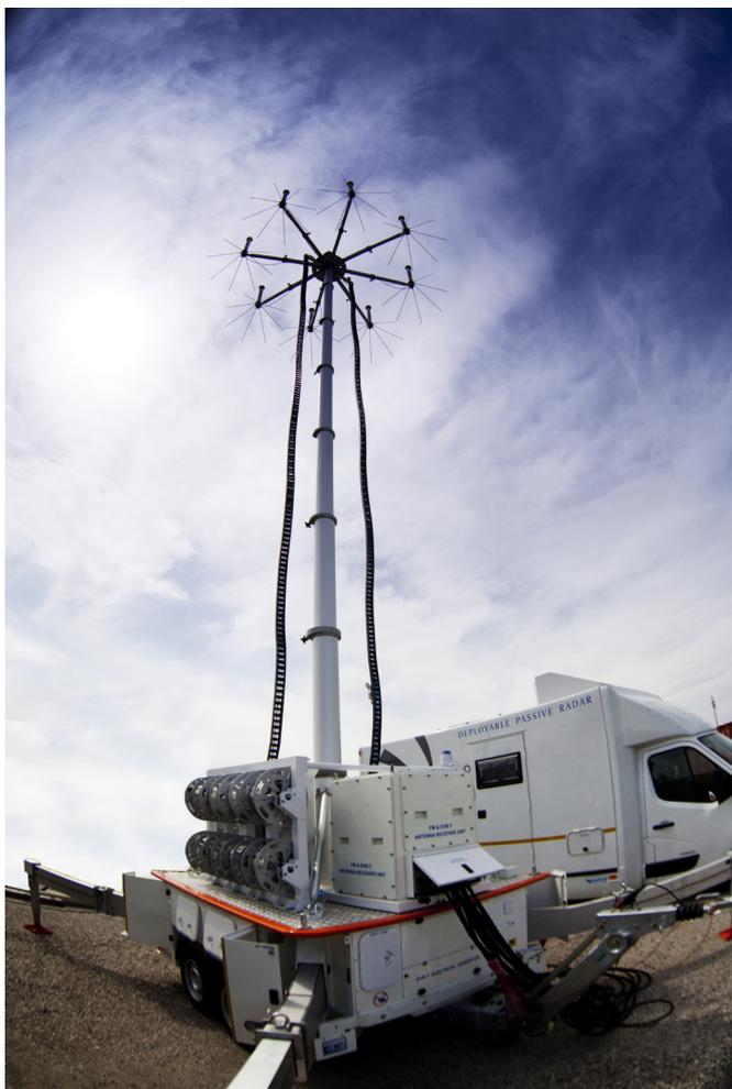
The system may be used for several applications, primarily for surveillance in many different missions. It can monitor the airspace around airports, ports and any element of critical national infrastructures. AULOS can also monitor commercial and military traffic up to a distance of several hundred kilometers.
