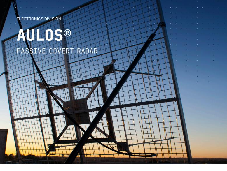
AULOS® is the passive radar system designed to provide detection and tracking capability for defence and homeland security applications. The system works by processing reflections from illumination sources such as commercial broadcast and communications signals. AULOS® is an ecofriendly system since it doesn't produce electromagnetic pollution.
