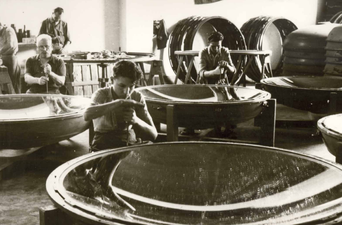
Mirrors being assembled – Officine Galileo, 1942
